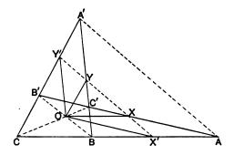
with the figure BCB'C'. If OX be drawn parallel to BC to meet B'C' in X, and if OX' be drawn parallel to B'C' to meet BC in X', it is evident that XX' will be that line of the figure B'C'BC which corresponds to the line at infinity in the figure BCB'C'. Hence the theorem is proved.
